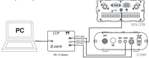
Fig. 2 Schematic Diagram of Connection Between DE-19 and G106C\XPA125B
